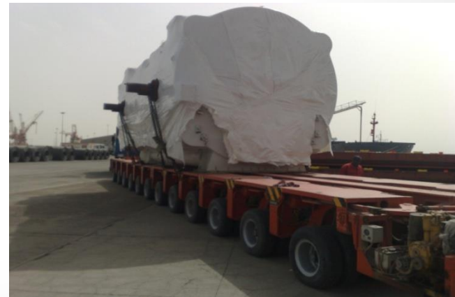
Turbine – 212 tons, 130 cbm, 1 piece
