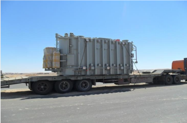
Transformers – 76 tons, 144 cbm, 24 pieces
