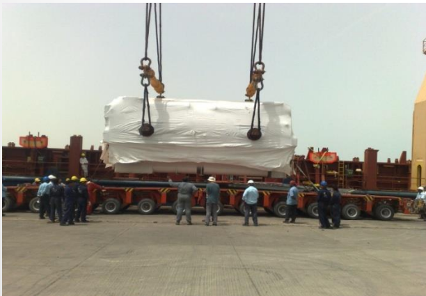
Turbine – 212 tons, 130 cbm, 1 piece
